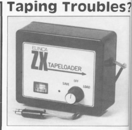
Elinca Products have announced the launch of a tape loader for use in helping you load and save programs to tape from the ZX81.
