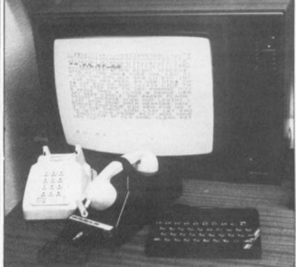
The Micro-Myte 60 acoustic modem, priced at £48.00, provides a low cost means of communicating information between compatible micros utilising the normal telephone network.
