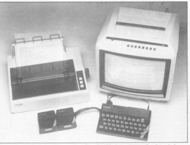
Here you can see the Spectrum connected to an Epson RX 180 printer, a letter quality printer, via the RS232 interface.
