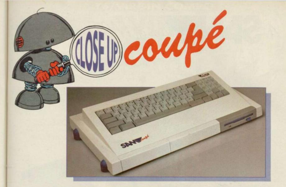
A 72 key full-sized, full travel **Keyboard**, designed with a professional feel. The keys are "soft", allowing you to re-program and re-position them if you wish. On the right, there are 10 function keys, which double as a numeric keypad.
