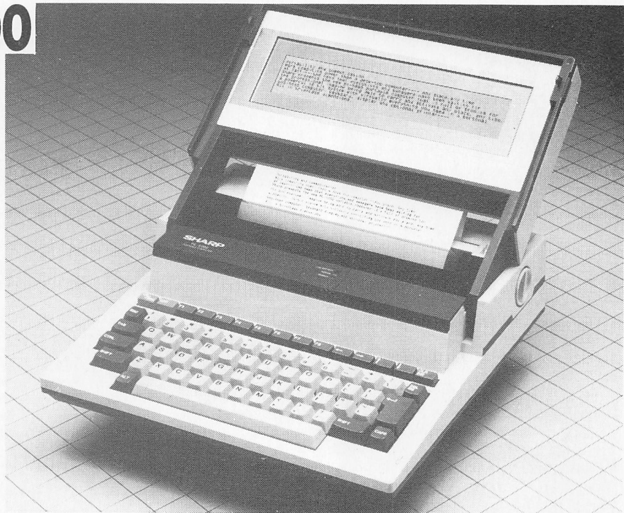
The Sharp PC-5000 is a powerful package featuring the unusual combination of standard MS-DOS operating system with bubble memory cartridges.
