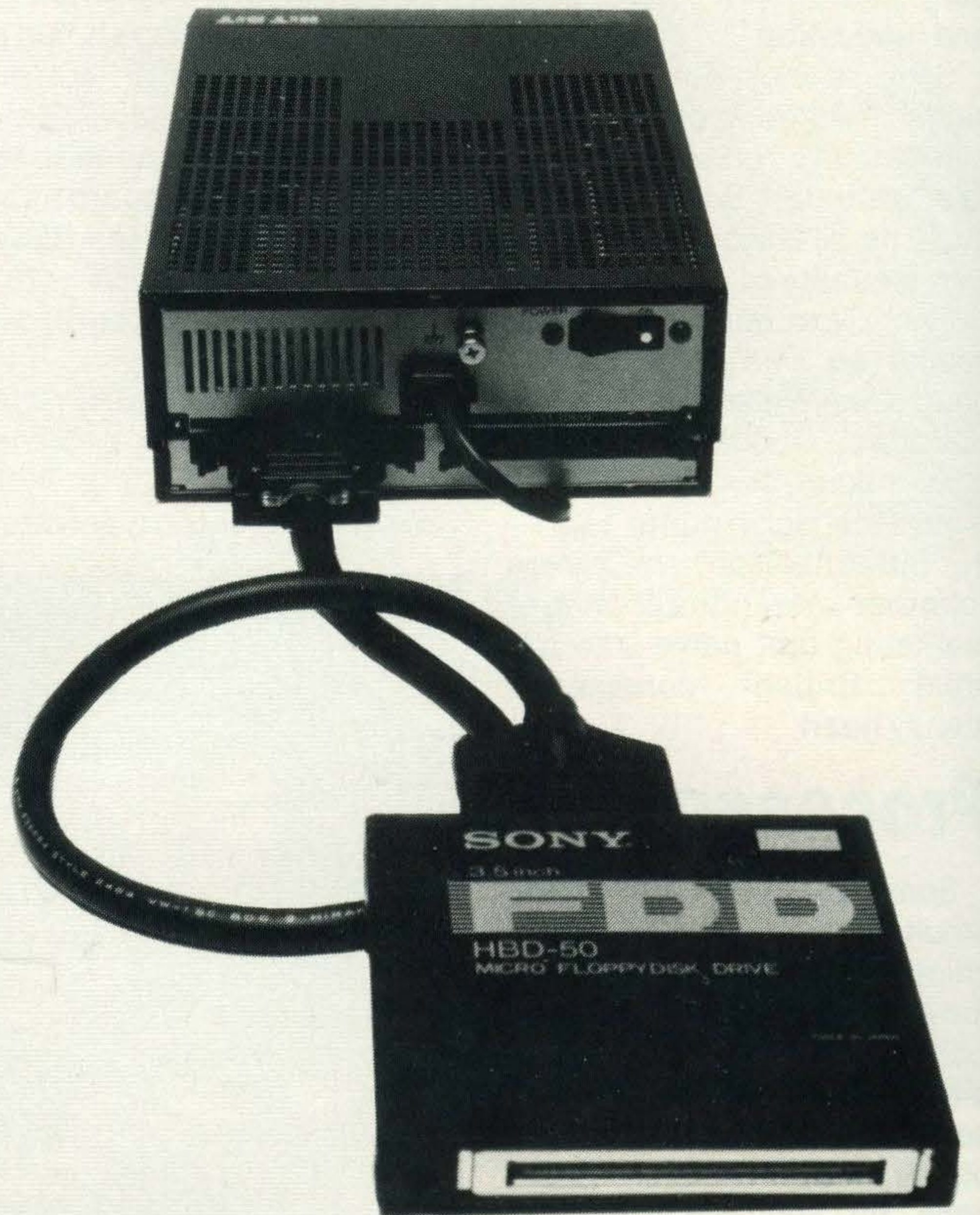
The disc drive interfaces via a special cable and cartridge. This plugs into the rear cartridge port
