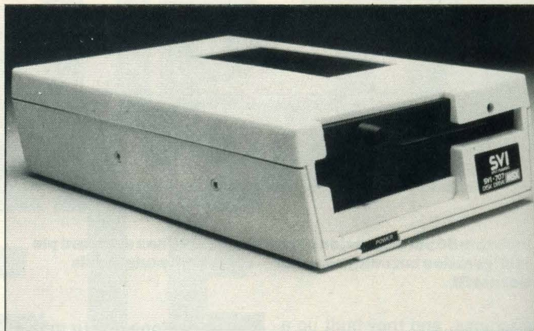
SVI-707 disc drive (£345) with built-in controller means CP/M is ready to run — If you have the 80-column card. Left — numeric keypad
