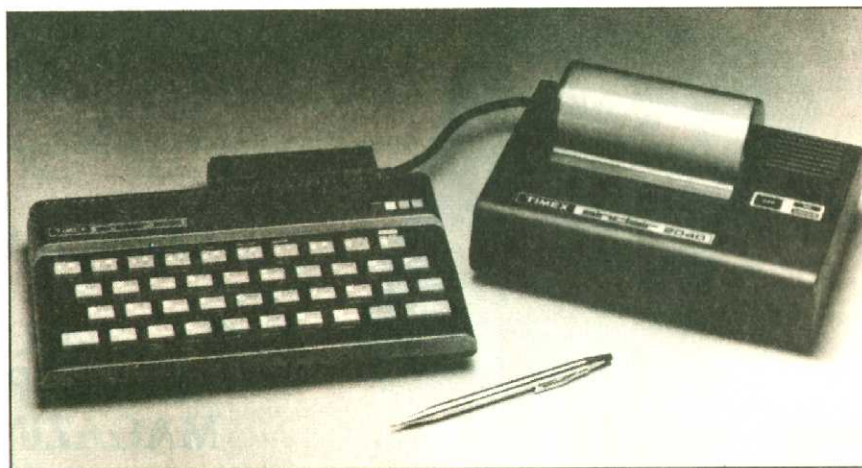
The Timex Sinclair 2000 and the 2040 thermal printer, which boasts full graphics and text capability, thirty-two column width, and a printing speed of two lines per second.
