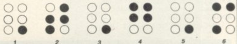
The characters 'TGM' in Braille. Grids 2, 4, and 6 represent T, G, and M; the grid used in 1, 3 and 5 shows that the letter following it is a capital.
