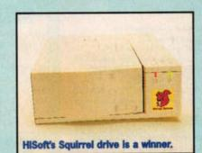
is lined internally with metal to form an electronic shield (this also applies to the Gasteiner and System Solutions drives). Firmly in the 'sandwich toaster' domain, this drive is light, fast and very easy to use. It comes with the ICD Link 2 SCSI interface and the excellent ICD software, so you can easily customise its partition layout.
