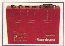
The FDI links the Falcon's DSP output with your DAT machine. Use it for dropping your mix on to DAT and for backing up your tracks.
