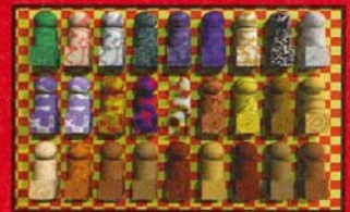
■ Texture mapping (wrapping pictures or patterns around an object) is the easiest way to give your models detail without actually needing to build it in. These are some of POV 's defaults.
