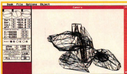
■ The camera mode, running on a Falcon. Here you set up the position of the objects and the viewing point.
