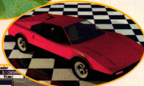
■ Place the camera in the 3D world of InShape using a system of X, Y and Z co-ordinates. Setting camera direction is as easy - enter the co-ordinate of the spot you want the camera to look at.
