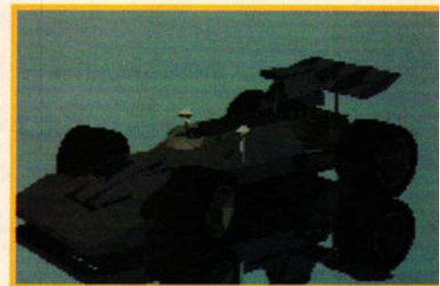
■ Our preliminary rendering of the racing car model saved as a 320x220 picture in "quick test" mode, it still takes almost two hours to generate this picture even if you're using the 68882 co-processor.
