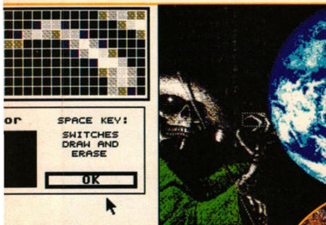
■ Left - The rather crude zoom function, you select the area of the picture from the full size section displayed on the right, a small zoomed section appears that you can edit. It is set at a fixed resolution and no drawing tools are available.
