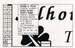
■ This is Silhouette's main work area, with GEM menus and graphic tools. There are three windows you can work in, you can't resize or move them but you can scroll around them. The Raster Window is selected and a Bit (Raster) image has been loaded into it for processing.
