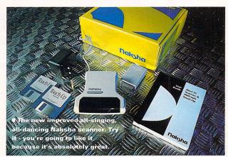
Naksha have launched a new version of their hand scanner for the ST with scanning resolutions ranging from 200 to 400 dpi. Included with the scanner is the powerful MiGraph *Touch-Up* package enabling you to alter and manipulate high
