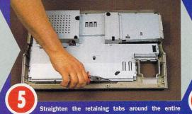
shield and remove the three screws that are positioned along the front edge of the machine.
