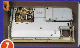
Remove the two screws holding the power supply to the base of the machine. These are located on the front left and front right support legs of the power supply.
