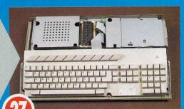
Plug in and replace the keyboard. The cable can only plug in one way around. Replace the top from the right side, ensuring the drive eject button goes into its slot. Keeping a firm grip on the machine, carefully turn it over and replace the screws
