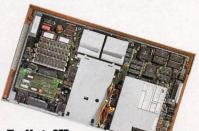
**The Mega STE** uses SIMMs (sensible) which are on the right-hand side of the machine. The 4MByte limit remains on the Mega STE range of machines.
