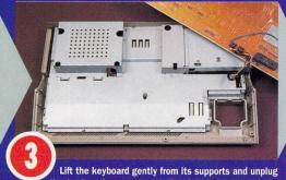
the keyboard connector at the right-hand side of the machine. Put the keyboard in a safe place.
