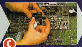
Insert the chip into the socket on the Video Shifter adapter, ensuring that it is the right way around as described in the installation instructions. Make sure that all the legs of the chip go neatly into the socket and they're not bent.
