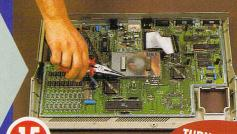
In the centre of the circuit board there is a large silver box, containing the Video Shifter chip. Using the pilers twist open the tabs that hold the lid down and open it up.
