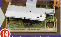
Remove the upper shield from the machine.
