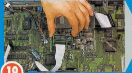
The main Shifter adapter can now be inserted into the socket on top of the shifter chip and firmly pressed down.
