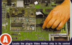
housing. Gently slide a small flat-bladed screwdriver between the bottom of the chip and its socket. Pry up the chip, ensuring that you do not touch or bend the legs of the chip. Some machines have a plug-in Video Shifter chip. Here the Zydec board is being installed on one of these. Follow the disassembly instructions as per the Xtra-RAM walkthrough steps 1 to 15.
