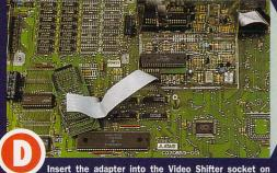
the main circuit board. Run the ribbon cable out towards the front of the machine and close the lid, ensuring that the cable does not get trapped or cut.
