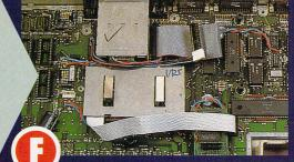
Plug the cable from the Shifter into the MMU adapter and the job is complete. Reassemble the machine as described in the Xtra-RAM walkthrough.
