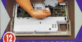
Remove the ribbon cable from the disk drive by gently tugging on it. It should disengage quite easily.
