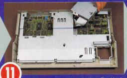
Lift the drive from its supporting legs. The drive is connected by a ribbon cable and a power cable. Note the position of the red core on the ribbon cable - it is usually at the front edge of the drive. The cable must be re-inserted the correct way! There is usually a lug which lines up the ribbon cable with the drive but it may be absent on some machines.
