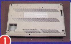
Turn your machine upside-down and remove the screws using the cross-head screwdriver. The screws in the square holes hold the lid on and the three screws in the round holes hold the disk drive in place. Store all screws safely. This is important because the screws at the front and rear of the ST are different lengths.
