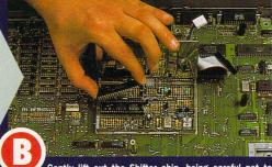
Gently lift out the Shifter chip, being careful not to touch the legs. Note this board has the non-standard oblong MMU and glue chips.
