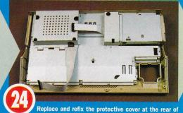
Replace and refix the protective cover at the rear of the disk drive with the ribbon cable running out, and replace and refix the power supply shield with the MMU cable running out as shown. Here the
