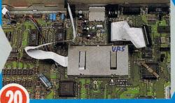
The lid to the Video Shifter housing can be closed with the ribbon cable running out to the left. Ensure the edges of the lid do not cut into the cable. Sometimes it's impossible to close the lid because of the extra adapter used with surface-mounted Shifters, so you have to remove the lid, using some snips to cut the hinges at the rear of the housing.
