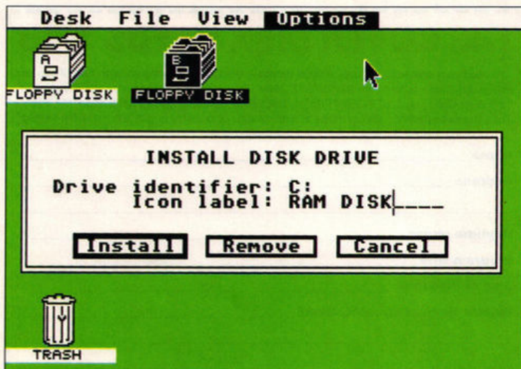
● Installing Drive C icon as a RAMdisk from the Desktop is as easy as – er, installing Drive C icon as a RAMdisk from the Desktop, really.
