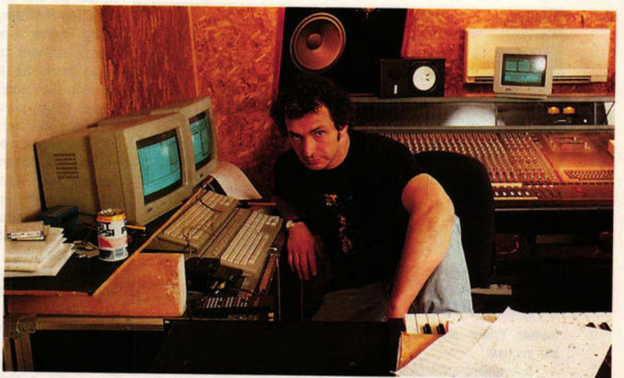
Big George stays patient, very nearly. On his left are two STs running Creator and Notator , while over his shoulder is the Mozart ST-based recording desk
