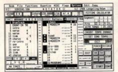
■ The elegantly laid out main menu of C-Lab's Notator showing 16 tracks, the Stop, Start and Record functions and the range of drop-down menus
