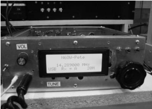
Figure 3 20m SSB Transceiver with Single DDS VFO
