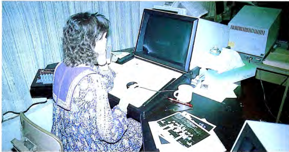
Above, manipulating the elements of a newspaper page is accomplished easily with a mouselike device. Below, the scanner digitizing artwork for input into the pagination system.
