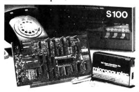
and answer. The Micromodem 100 comes with the Microcoupler and is fully S-100 bus compatible including 16-bit machines and 4 MHz processors. The Micromodem 100 operates at either of two software selectable baud rates — 300 baud and a jumper selectable speed from 45 to 300 baud.
