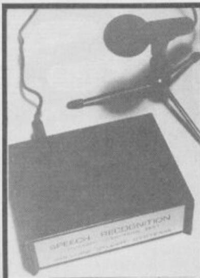
spoken commands through the I/O port. For instance, you could teach Big Ears 'left' and 'right' and write a Basic program to link those words to the movement of a floor turtle or similar robot.
