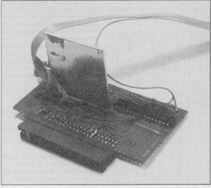
but there are a few things to watch. First, all the metal surfaces must be clean and free of grease or corrosion. As you'll be using new bits, that shouldn't be a problem. Second, there's the technique.
