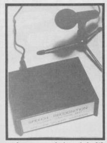
spoken commands through the I/O port. For instance, you could teach Big Ears 'left' and 'right' and write a Basic program to link those words to the movement of a floor turtle or similar robot.
