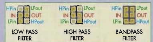
Fig.8: follow this parts layout diagram to build the PC board. The various tables show the values for resistors Ra & Rb and for the filter components (R1-R3 & C1-C2), while the linking options for the selection matrix are shown at right. Links LK1 & LK2 go in position 1 for a dual-rail supply (or for an AC supply) but must be moved to position 2 for a single-rail supply.
