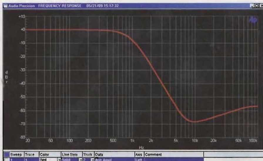
Fig.5: this screen grab shows the frequency response for the low-pass filter configuration with a nominal corner frequency of 1kHz. The attenuation slope is 24dB per octave.
