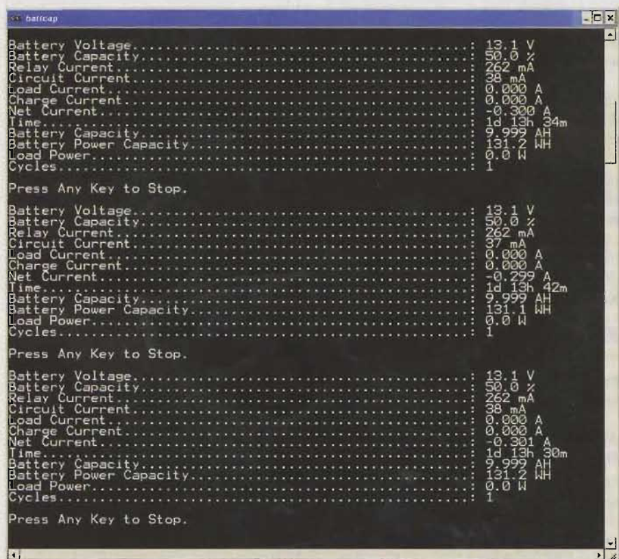
Fig.13: this shows the result of running the command line "battcap.exe -x" – the real-time readings are displayed every second.
