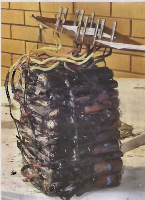
The plug-in capacitor box contained a large number of faulty paper capacitors, which meant that a complete new assembly had to be made up.
