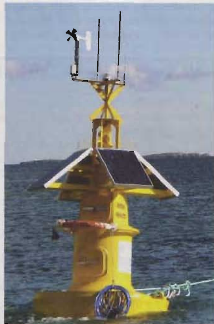
Monitoring buoys are used to monitor salt concentration, dissolved oxygen and many other parameters. If these exceed safe levels the desalination plant will be shut down until the ocean currents can return the sea water to acceptable levels. (courtesy Water Corporation)
