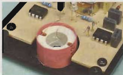
A close-up of the coil (L1). It's about 400 turns of wire on a plastic bobbin.
