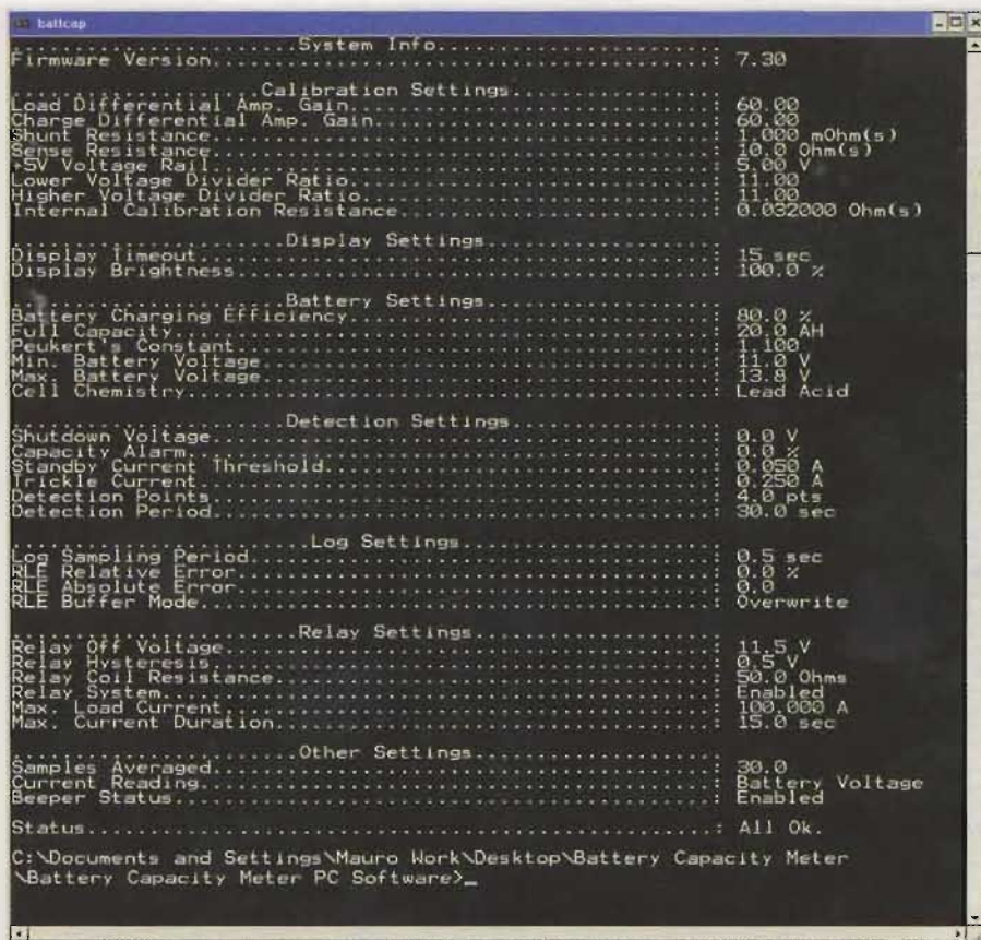
Fig. 12: a screen grab showing the result of running the command "battcap.exe -i" to get information on the current settings.
