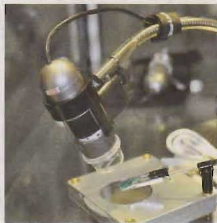
Scinet’s Dino-lite handheld (or in this case stand-held) USB microscopes.
