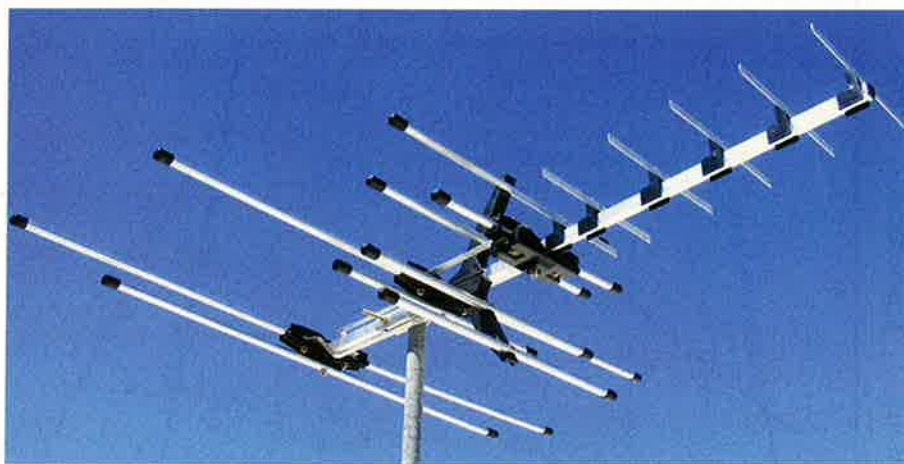
This digital-only combined VHF/UHF Yagi from Hills is so new it's not scheduled to go into production until next month! Note the quite short VHF elements on the rear of the antenna - short because they don't have to pick up the low frequency (and therefore longer wavelength) VHF channels which are analog-only. The short UHF elements are on the front of the boom in front of the driven element and corner reflector.
