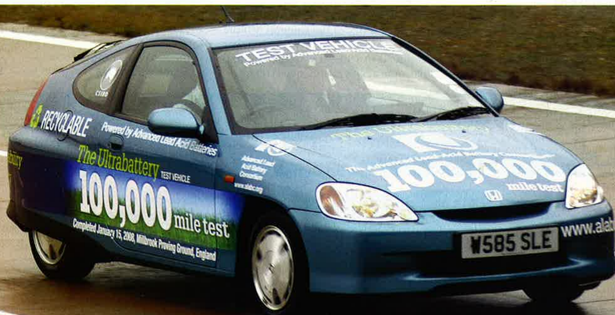
A hybrid test car on a test track in England, powered by the CSIRO-developed UltraBattery – a combination of an ultracapacitor and lead-acid battery. Photo courtesy Advanced Lead-Acid Battery Consortium.
