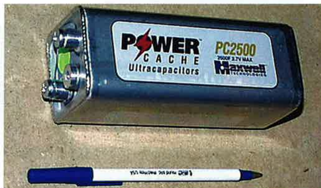
A 2500F (or 2.5kF) Maxwell Power Cache Ultracapacitor. Note the low operating voltage (2.7V) – this means that many of these must be used in series to obtain any type of reasonable voltage rating. The photo at right shows the same capacitors installed in a Honda EV conversion. (Photos courtesy www.metricmind.com ).
