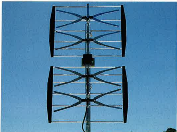
Examples of horizontal (left) and vertical (right) polarisation on this Matchmaster 02MM-MDU36 4-bay phased array (also known as a 4-bay bowtie) antenna from Jaycar Electronics. We have to say it's one of the better-made digital TV antennas we have found – so good, in fact that it sits on a short mast on top of the SILICON CHIP offices, aimed at the North Head repeater.
