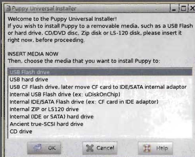
Fig.3: you can install Puppy on both internal & external disk drives. It can even go on a compact flash (CF) card that's fitted to an IDE adaptor and substituted for the hard disk drive.
