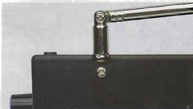
Here's how the pitch antenna mounts: a small cutout in the case lid allows it to be mounted to the side of the case via the screw clearly visible in this photo.
