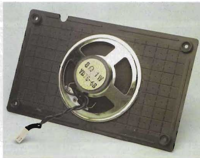
The internal speaker is secured to the lid with silicone sealant or other suitable adhesive.
