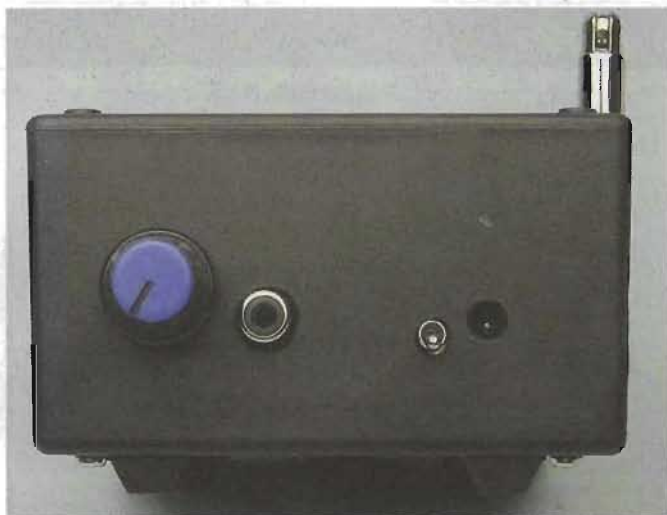
The control end of the Theremin – from left to right the volume control, line output socket, power switch and 12V AC power input.
