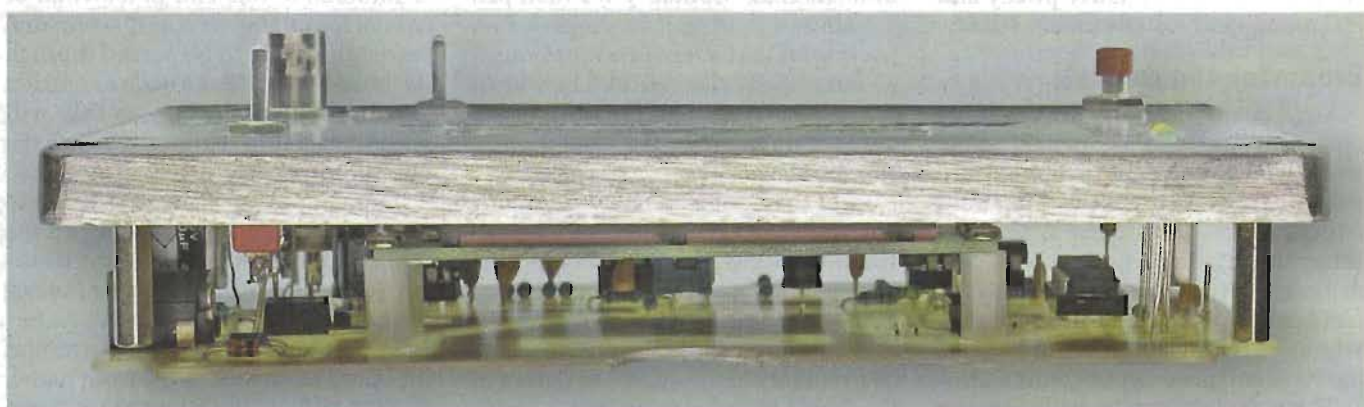
Fig.6: the PC board is attached to the lid of the case via four M3 x 25mm tapped spacers as shown here. Four M3 x 6mm countersink-head screws secure the lid to the spacers, while four M3 x 6mm pan-head secure the PC board.
