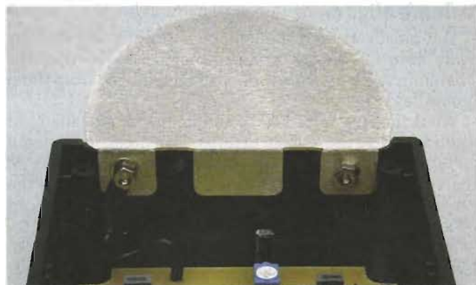
Looking inside the open case, this photo shows how the volume plate is secured.
