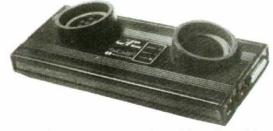
An example of an accoustic modem. Note the rubber cups where the telephone handpeice fits.
