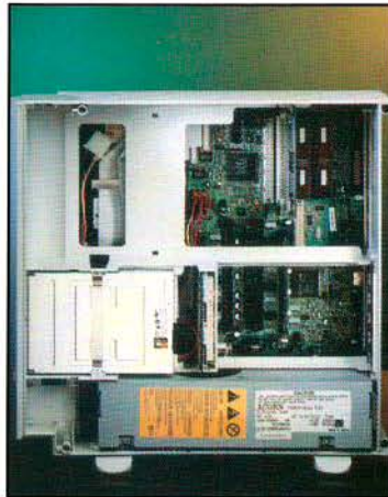
Figure 2. A basic system with single 'slice' containing floppy disc drive fitted over the tray containing motherboard, power supply and hard disc
