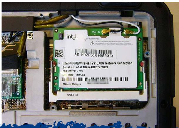
*Placa wireless Intel 2915ABG mini-PCI instalada*
