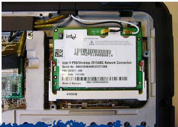
*Placa wireless Intel 2915ABG mini-PCI instalada*
