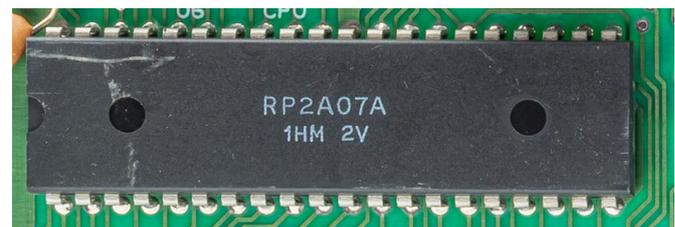
Fig. 8 - The CPU produced by Ricoh for the Famicom/NES, here PAL version (author: PantheraLeo1359531 - source: Wikimedia Commons)
