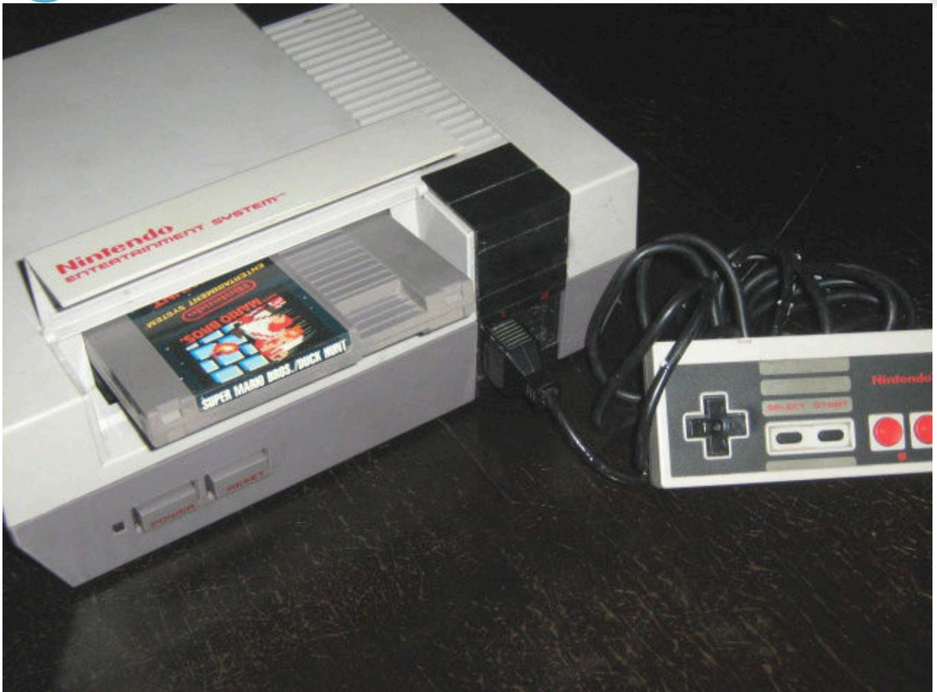
**Fig. 11 - The loading of cartridges on the NES was designed to resemble that of videotapes in epopca VCRs (author: Yagamichega- source: Wikimedia Commons)**
