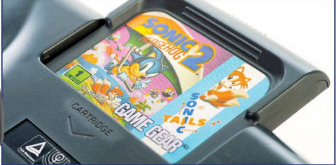
» Game Gear cartridges are compact and feature a pronounced ridge, allowing easy removal from the system.
