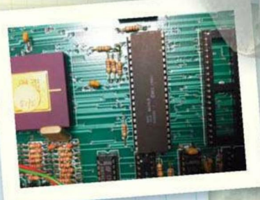
The Konix chip is labelled in yellow, the central chip shown is the NEC 8088 CPU
