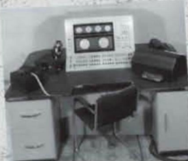
THE MARK I'S OPERATOR CONSOLE, SHOWING ITS CRT BASED MEMORY BANKS.
