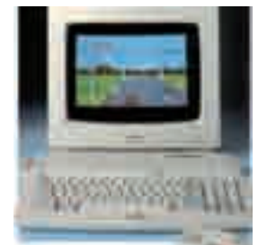
» A new case and the addition of a cartridge slot – for expensive £30 games – transformed the 464 into the 464 Plus
