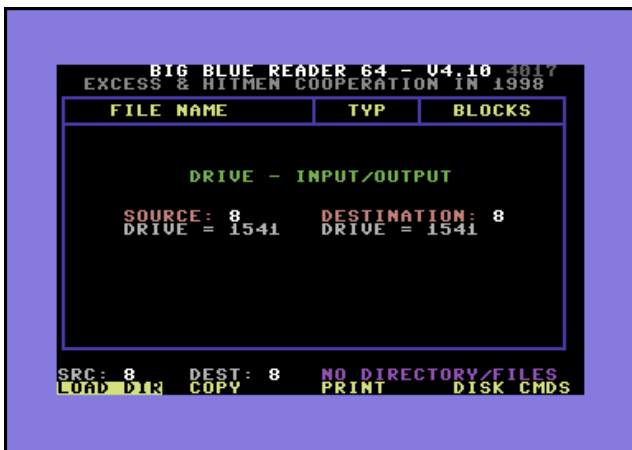
Big Blue Reader allows you to transfer your Commodore Documents onto PC as a text file.
