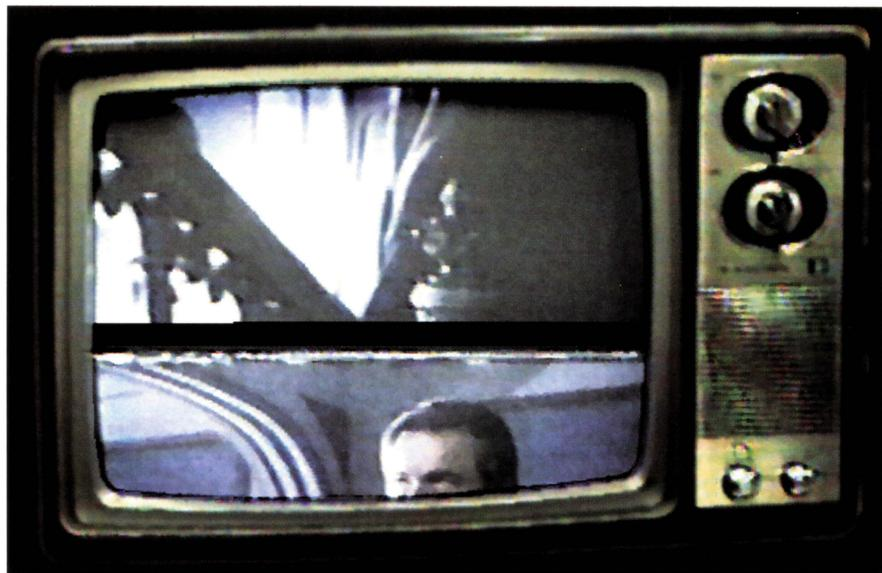
At top, by adjusting the vertical hold, you can see the "missing" lines of the picture. Bottom, a close-up of the closed-captioning data that's transmitted along with the picture.
