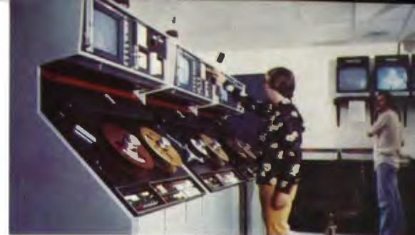
Quad tape complement at TV-8 includes three TR-600A machines, each equipped with AE-600 Time Code Editing Systems, plus a workhorse TCR-100 "cart" machine.
