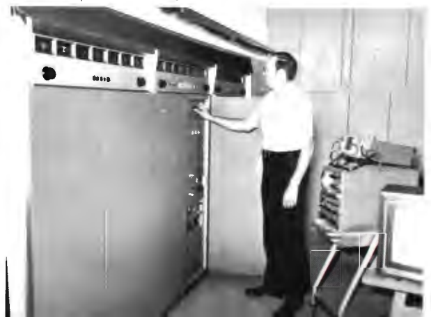
Tall Transmitter Supervisor Frank Kresl with TT-50FH parallel transmitter. The 50 kW transmitter, remote-controlled from the studio, operates around the clock, and has logged an excellent performance record.
