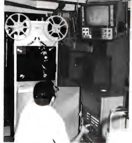
Waveform monitor below picture monitor simplifies adjustment and maintenance for TK-28. A mirror arrangement permits MC operator to keep TP-66 film reels in view to verify upcoming commercial breaks in film shows.
