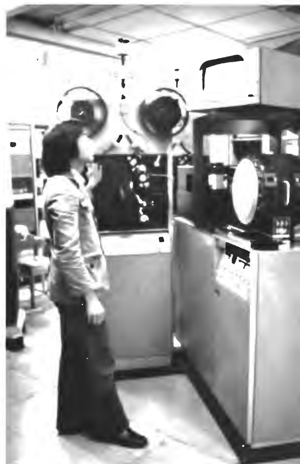
Five telecine systems, including this TK-28 with ASCET, are kept busy transferring English-language film programs to tape.
