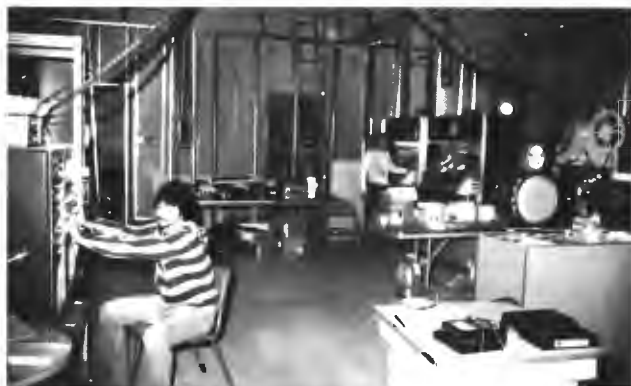
Addition of a TK-28 telecine island and two TR-22 VTR's moved TV-4 into full local and network programming and commercials.
