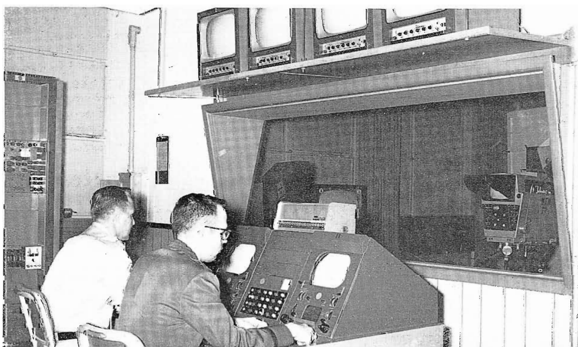
FIG. 28. TK-60 camera controls, film remote control and master monitors in Studio B control room.
