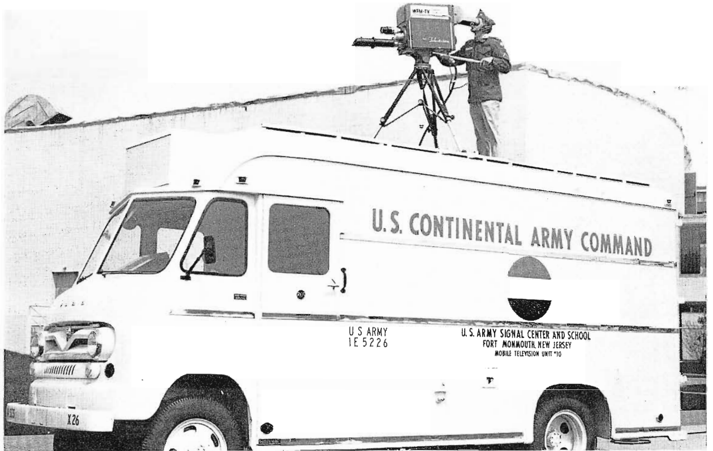
FIG. 2. Mobile van with cameras, TV tape and microwave link makes remote pickups for instruction and troop entertainment.
