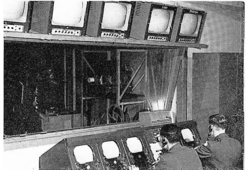
FIG. 23. Video engineers at control console observe pictures on camera controls and overhead monitors, perform switching.
