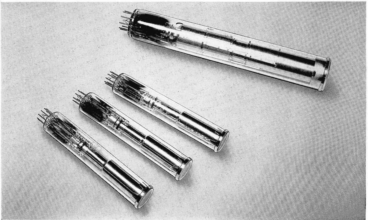
FIG. 2. Four tube principle . . . Three one-inch vidicon tubes are used in the red, blue, and green channels to provide the color (chrominance) signal. A 1½-inch vidicon is used in a separate channel to provide the monochrome (luminance) signal.
