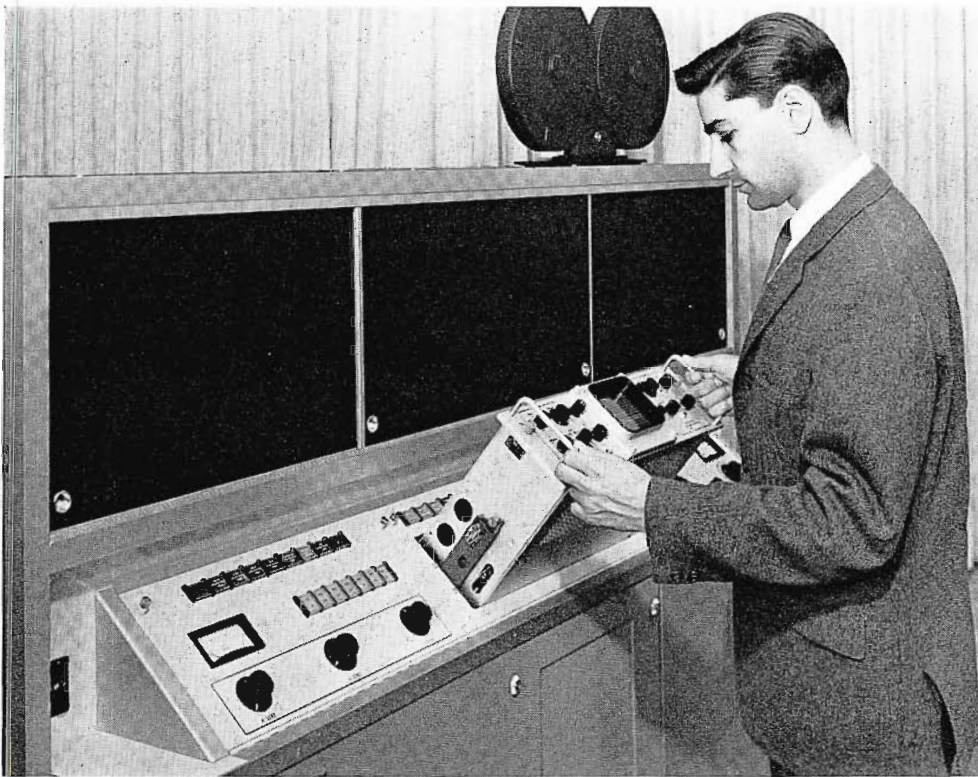
FIG. 5. Engineer demonstrates easy removal of waveform monitor. Complete accessibility of all components and circuits is a feature of the TFR-1.
