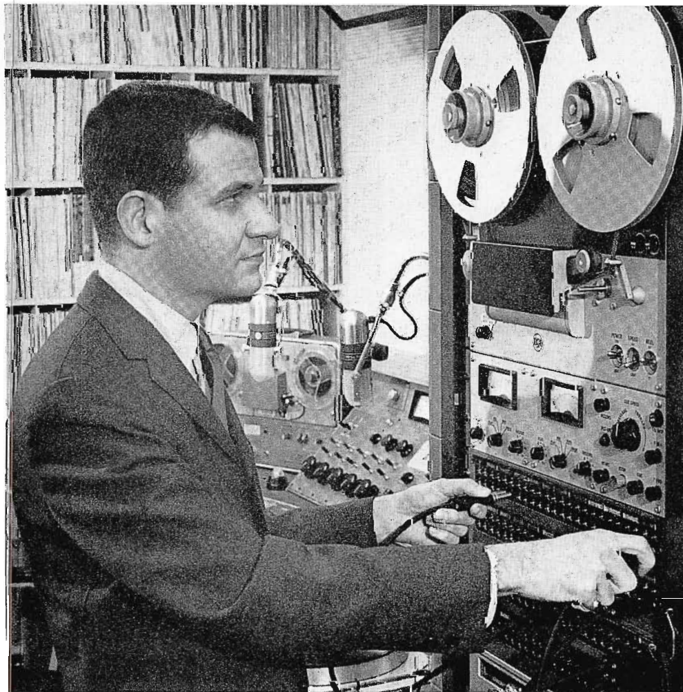
FIG. 3. KRAV President George R. Kravis makes a change in the audio patch panel. Recorder at top is reel-to-reel RT-21A. The cartridge-tape devices, Type RT-7, are immediately beneath the patch panels.
