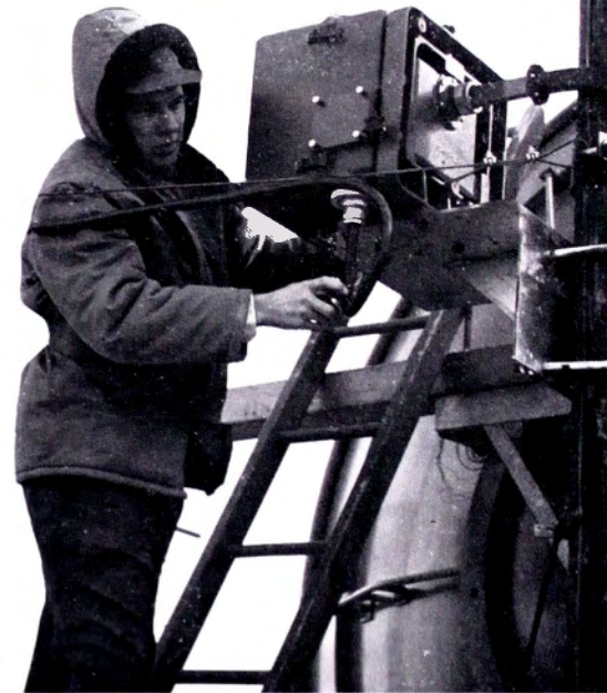
FIG. 2. Carroll Secrist, Chief Engineer, KID-TV, makes last minute adjustments to TVM-1B microwave receiver at the Albion receiving location.
