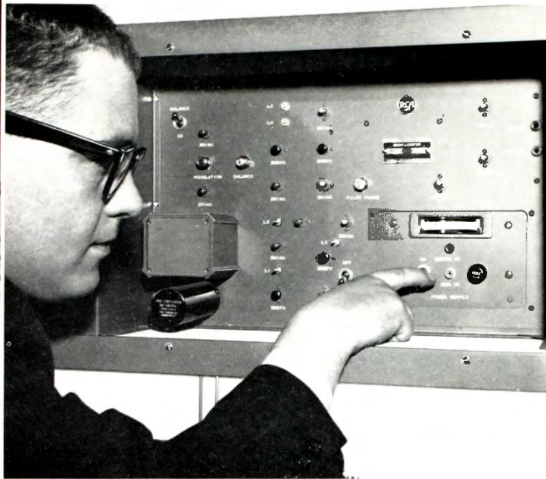
FIG. 5. Sum and difference signal transmission for the new FM stereo system is easily accomplished with the new RCA stereo generator. This compact all-transistor unit generates the supersonic double sideband suppressed carrier AM signal that contains the stereo difference signal. The main channel FM signal is the sum of the two stereo channels, and for receivers not equipped for stereo it sounds like a normal monophonic signal.
