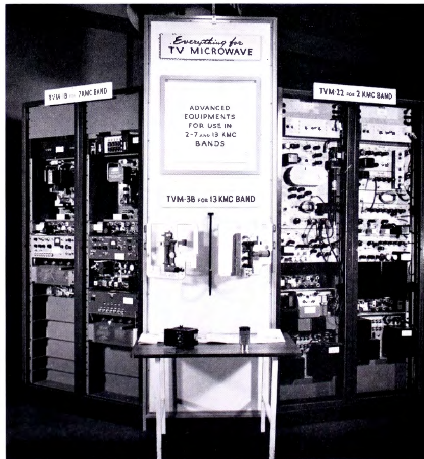
FIG. 13. Exhibited here is everything for TV microwave. Two new systems; one for use on 2,000 megacycles, another for use on 13,000 megacycles, round out a complete RCA TV microwave equipment line (including the 7000 megacycle equipment, Type TVM-1B).
