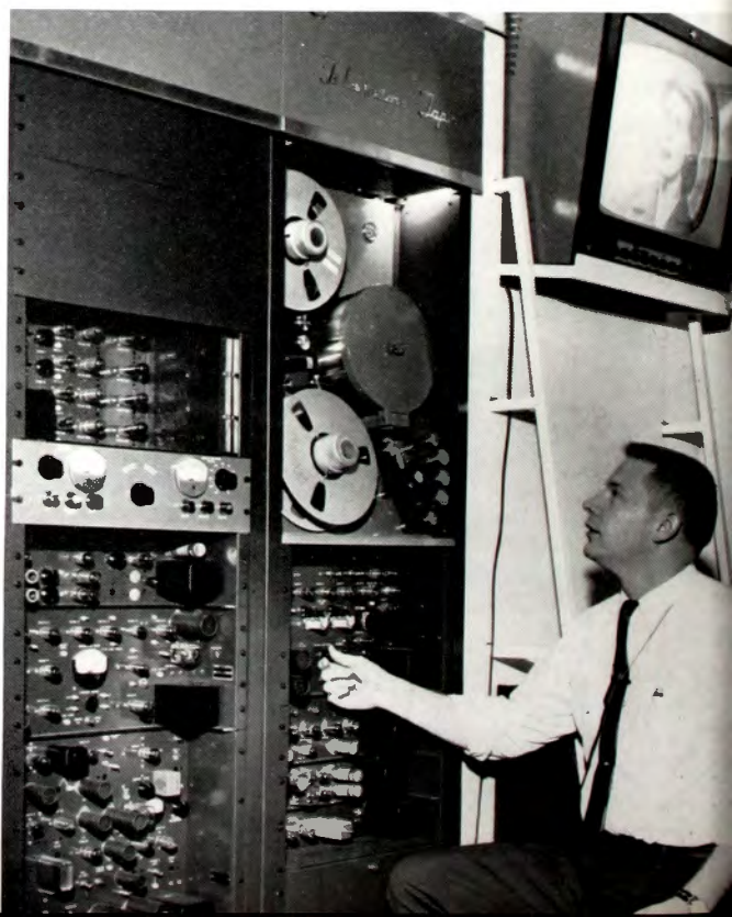
FIG. 2. New Slant-Track Closed Circuit Recorder, MR-700. Using a different principle from the other recorders in the family, this recorder records information on slant angle across the tape. Only two recording heads are used. Tape speed is cut in half—thereby using only half as much tape to record.
