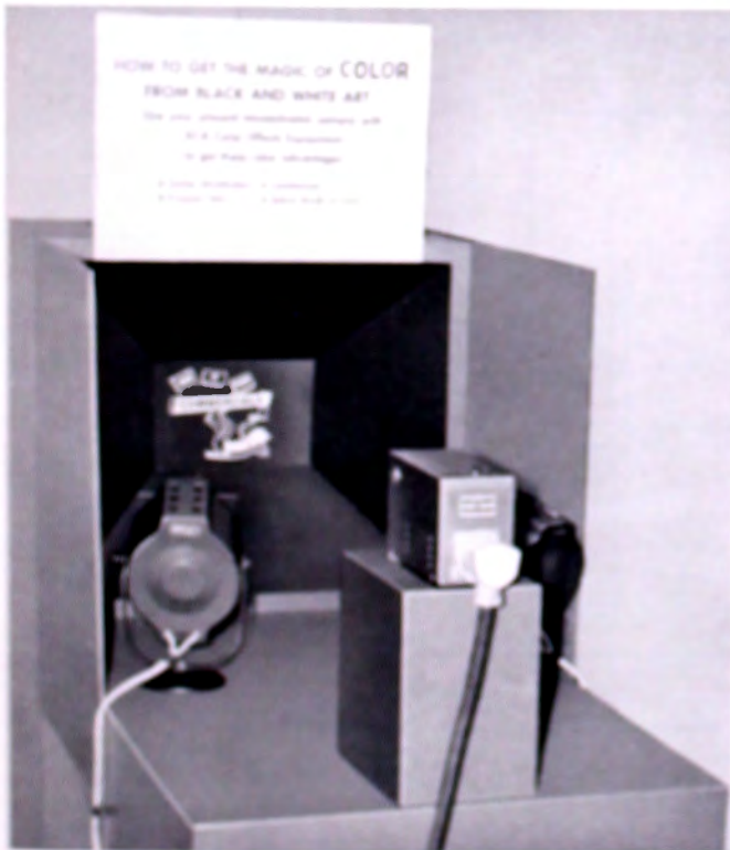
FIG. 3. For demonstration purposes, this combination of show cards and TK-21 Camera was used. The TK-21 may also be used normally with slides and opaques, or a live studio camera can be used with flip cards.
