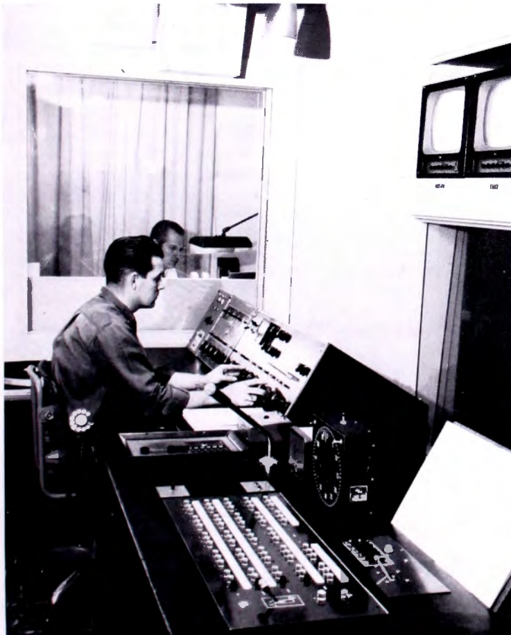
FIG. 17. Sub-control A. In foreground is a panel for TS-40 Switcher. Joe McCrady is operating BC-3 Console. In background is announce booth A.
