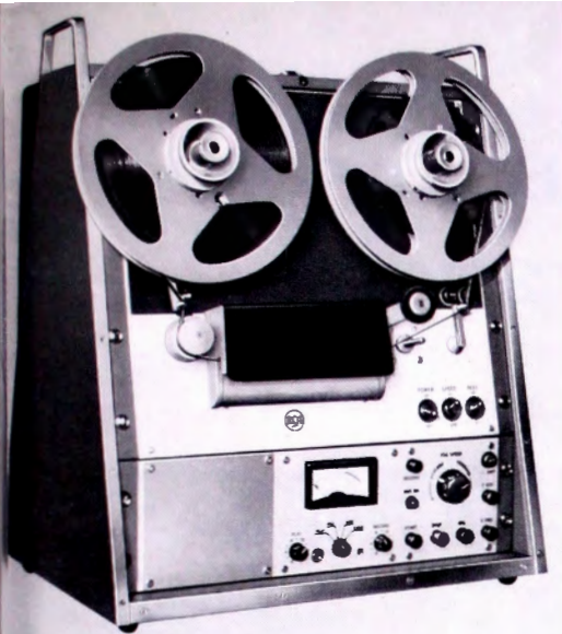
FIG. 3. Mounted in this rugged carrying case the RT-21A can be used for recording at remote locations or it can be easily moved within the station.
