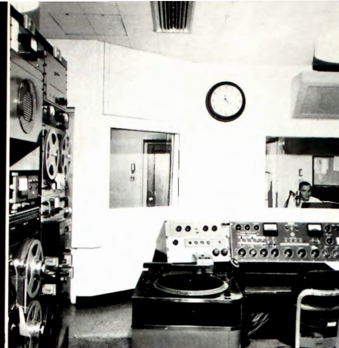
FIG. 19. Radio master control, showing BC-6 Dual Console. Announce-control room is seen through window.
