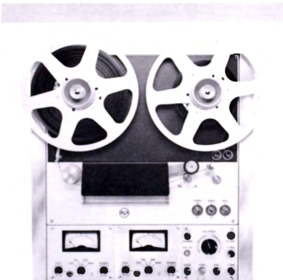
FIG. 1. This is the stereo version of the RT-21A Tape Recorder with two record/play amplifiers mounted side by side. The control unit is on the right. The tape transport unit (above the amplifier panel) is very functional. Straight line tape threading is accomplished without disturbing the head cover.
