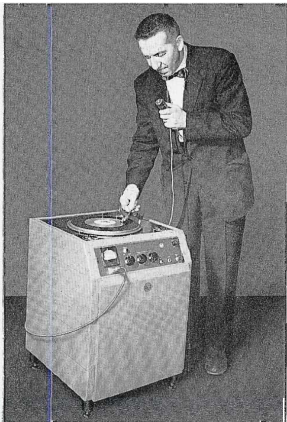
FIG. 9. Magnetic discs are easily recorded. The convenient microphone jack is just below the meter on the BA-51A Record/Reproduce Amplifier.
