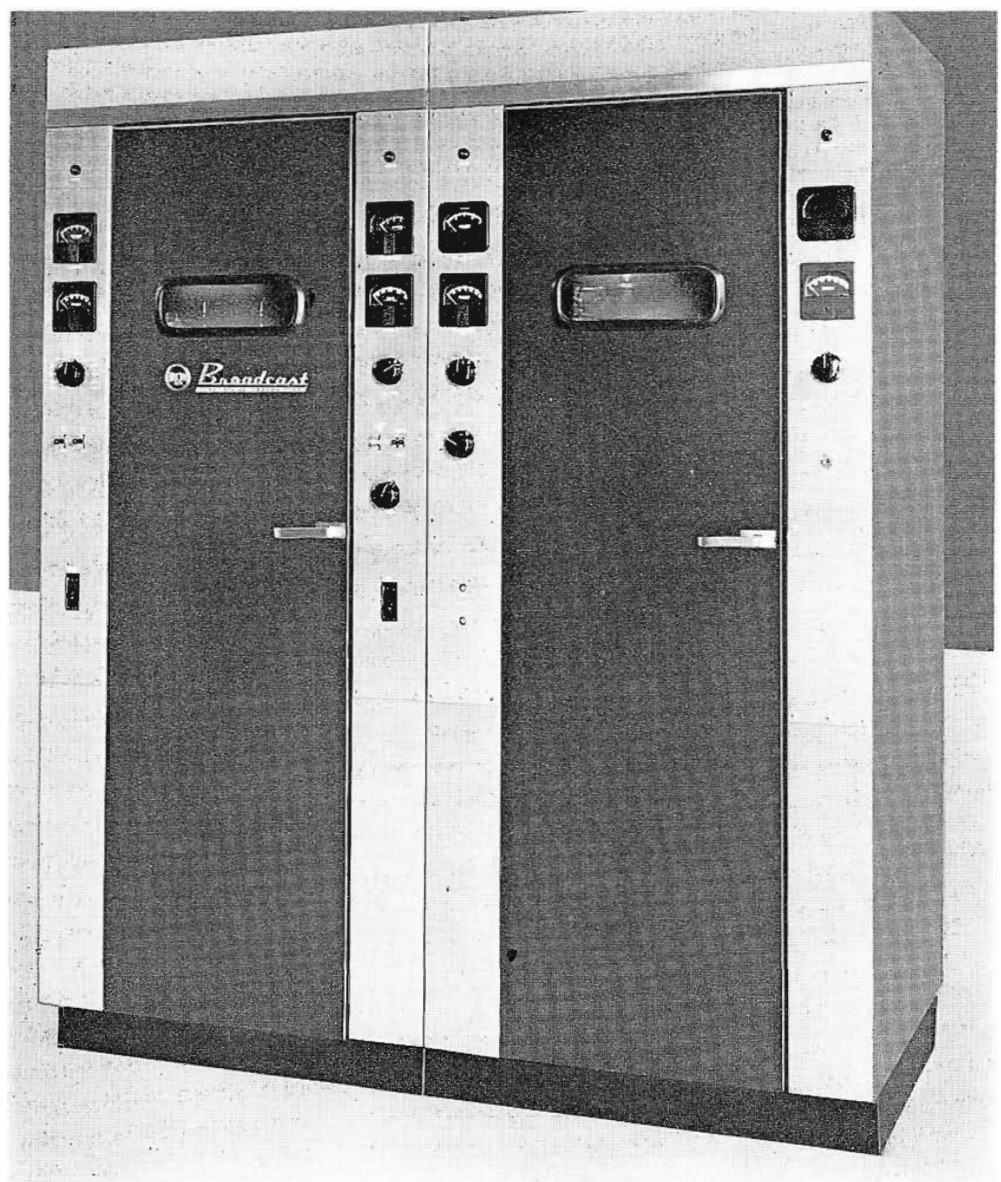
FIG. 1. Front view of BTA-5R. Easy access to all tubes and operating controls is made through the two interlocked front doors. The PA, modulator, and rectifier components are in the cabinet on the right, and the exciter, IPA, and control equipment are on the left. Attractive aluminized-steel cabinets provide improved shielding, and the doors are available in a choice of red, green, blue, or gray finishes.
