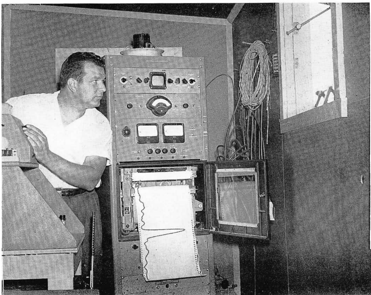
FIG. 9. As patterns of the antennas are measured they are continuously recorded as shown here. The speed and rotation of the turntables are also controlled from this location.
