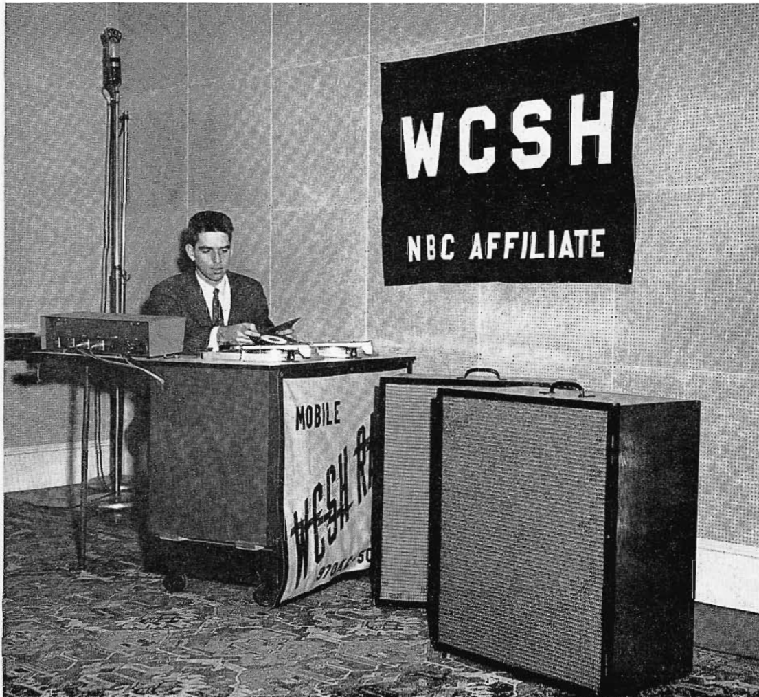
FIG. 1. This is the remote setup used by WCSH. The BN-6A Remote Amplifier, two turntables, and a public-address amplifier are in the large "box" on wheels which also serves as console desk for d.j. Two separate speaker enclosures are shown at the right.
