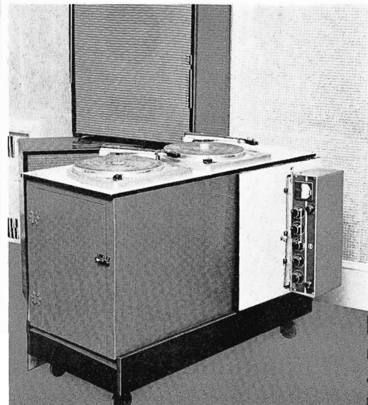
FIG. 3. The BN-6A Remote Amplifier is easily dropped into this position when moving the remote setup.
