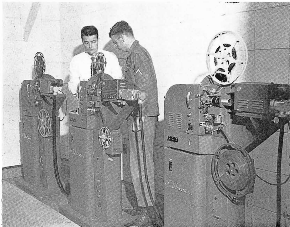
FIG. 5. Telecine with RCA film vidicon cameras and 16-mm projectors showing RCA Field Engineer, William G. Bedsole, and Pfc David H. Chute, telecine operator, adjusting projector.
