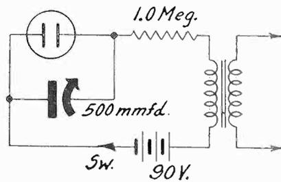
Intensity control is exercised at left by flipping the switch. The frequency remains practically unchanged. At right a variable condenser is used, for wide frequency change. The tubes must be of the type without limiting resistor built in.
