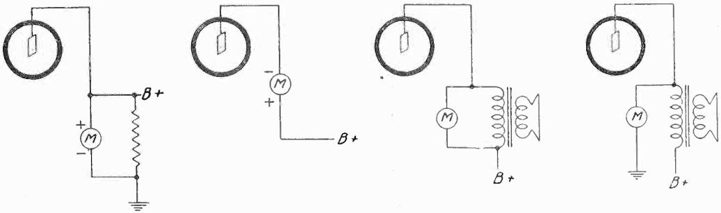
A meter is put in parallel with a voltage for measurement, but in series with a current. Left, meter B plus to ground; next milliammeter in series with plate; next two, voltages. D.c. voltmeters here would not measure a.c. But some a.c. voltmeters would be actuated by d.c. as well as by a.c.
