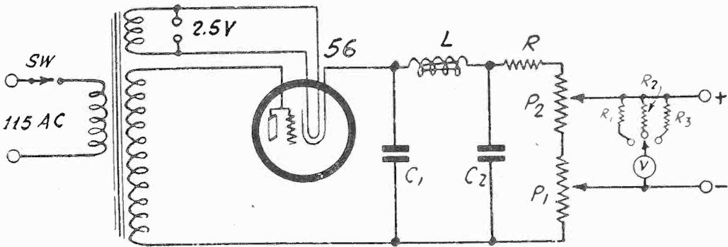
If batteries prove annoying in resistance measurements, use a simple rectifier. The voltmeter will read the voltage, which will not change when the sensitive milliammeter is used for resistance measurements at plus and minus at right, with proper limiting resistors. The same meter used for resistance measurements may be the voltmeter V. Extremely high resistance may be read, due to the high voltage 50 meg., easily.
