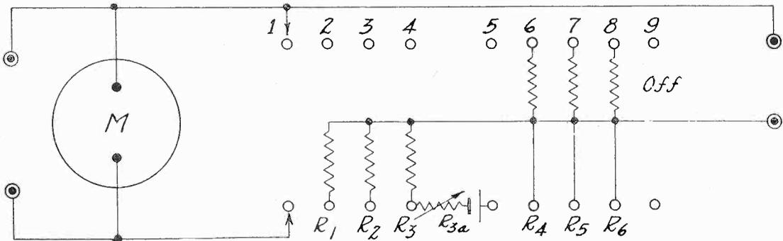
Direct access to the meter is at posts at left, for 0-1 milliamperes, or for low resistance measurement when the switch is at position 5 and the right hand posts shorted for full scale deflection.
