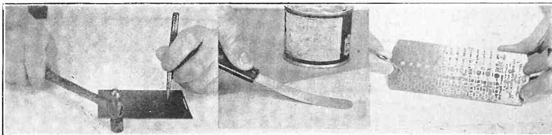
Many a small hole need not be drilled in soft metal. Save time and effort. Use nail punch (not center punch, which has sharp point, or once did have). Center instrument levels ridges for restoring console finishes. Template at right receives drills, classifies them, reveals how to use them, but not how to stop neighbors from borrowing them.
