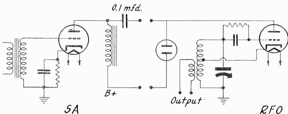
The left-hand tube is the output of a speech amplifier and the audio frequencies are put into a neon tube, which acts as a closing relay to apply plate voltage to the radio frequency oscillator RFO.
