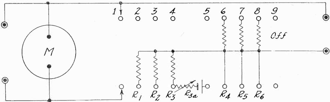
Direct access to the meter is at posts at left, for 0.1 milliamperes, or for low resistance measurement when the switch is at position 5 and the right hand posts shorted for full scale deflection.
