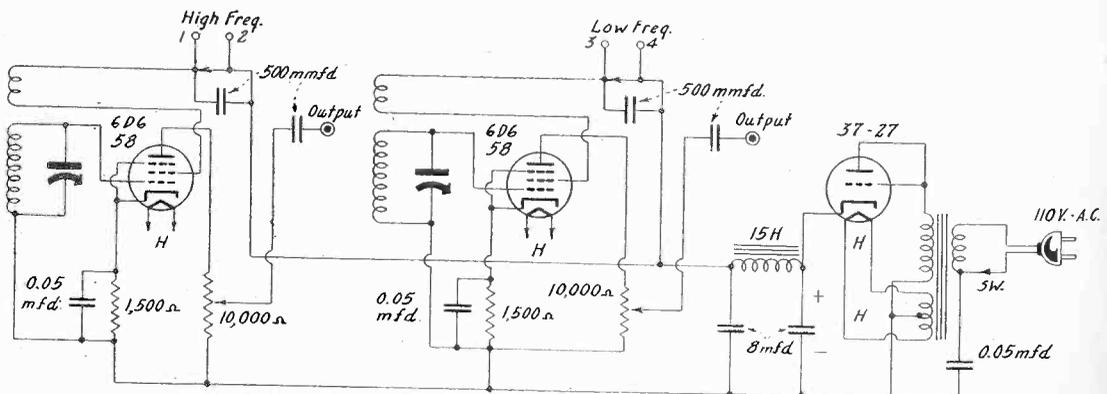
Put earphones between jacks 1 and 2 to listen to short waves or measure the frequencies of short waves when the broadcast oscillator at right is going. Put earphones at 3 and 4 to hear broadcasts, or to measure frequencies of still lower frequency oscillators.
