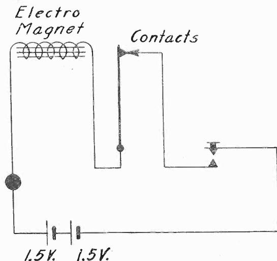
Circuit diagram of the buzzer and standard flashlight dry cells. Two cells used to supply the necessary energy. Depressing the key closes the circuit electrically, causing the electro magnet to become energized, which in turn pulls over the armature which breaks contact, thus opening the circuit again and armature returns to normal position, closing contacts. The cycle is repeated rapidly, thus resulting in the familiar buzzing sound.
