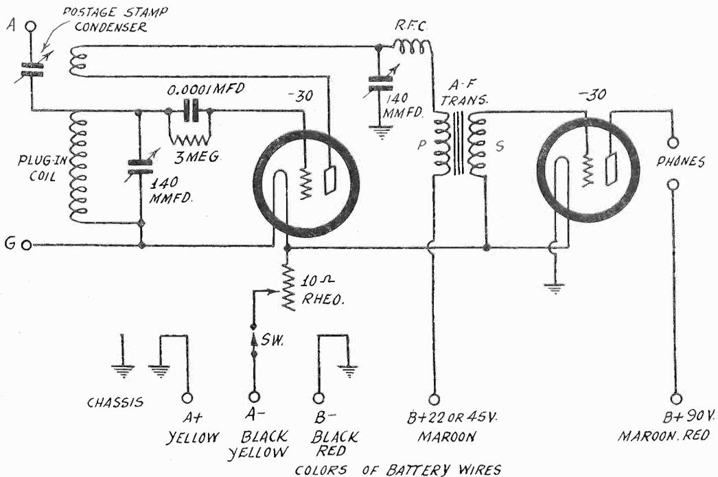
The tapering parallel lines used as ground symbol also are used as chassis symbol under conditions where chassis may or may not be grounded. To avoid any confusion the meaning of the symbol as used in a particular diagram is given, thus symbol above means chassis. That chassis in above example is not grounded is evidenced by negative filament going to G (ground).
