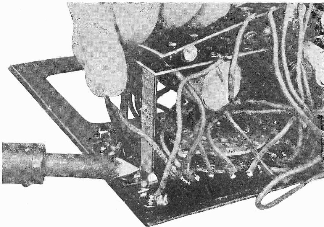
The final joint is being soldered at a binding post. The switch must be carefully wired and soldered.
