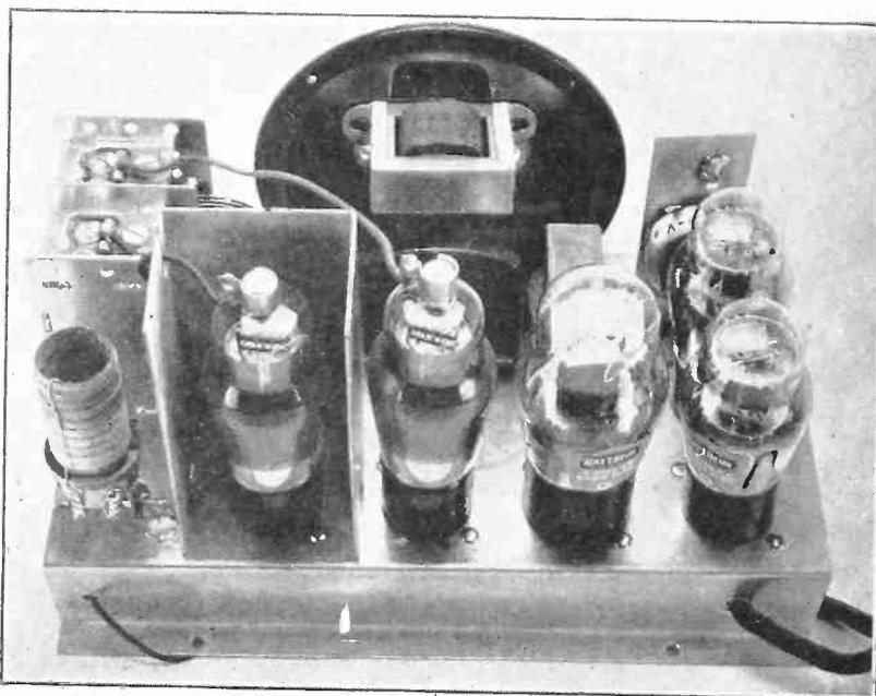
The two-gang condenser and the two coils provide sufficient results to give regular local reception amid trying conditions to selectivity and also afford some distance reception. The circuit diagram at right was built into the chassis in the form shown at left, the antenna coil being at the top, and the interstage coil (not shown) at bottom. The 200 ohm 50 watt resistance is connected to the line cord.
