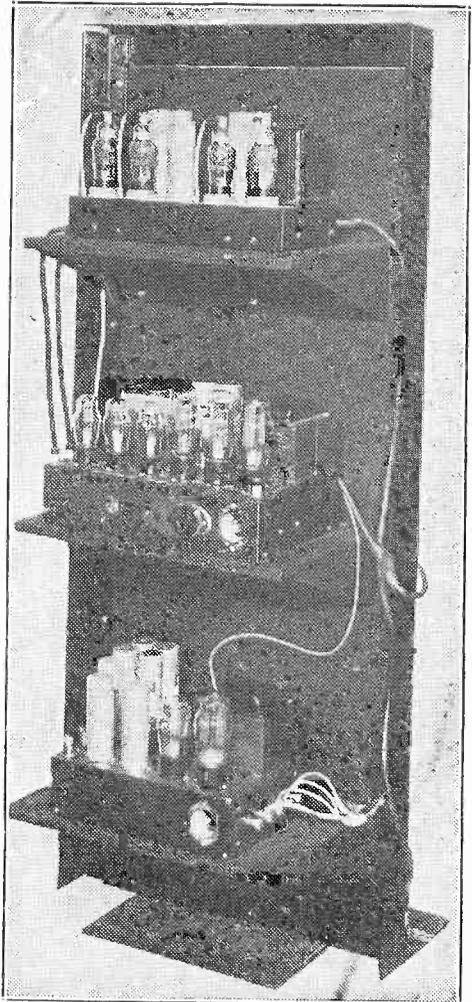
Many persons, after getting hookups to work well, like to set up their rigs in suitable containers. The rack and panel method of construction is growing in its popularity because of its professional appearance as well as all-around suitability, except for parlor, bedroom and bath. A microphone pre-amplifier, a power amplifier and a speaker field exciter are shown (top to bottom).
