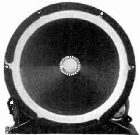
Front view of the Rola chassis. Holes are provided for attachment to your own baffle. The rim is protected by a lining of felt. The voice coil (center) is firmly mounted.
