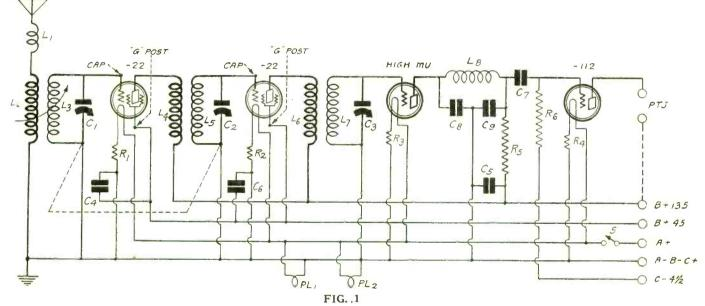
THE HIGH MU TUNER FOLLOWS THE GROWING PRINCIPLE OF OBTAINING STILL HIGHER SENSITIVITY AND VOLUME, WITH FEWER TUBES, DUE TO THE HIGH AMPLIFICATION CONSTANT OF THE NEW TUBES EMPLOYED. THE RF AMPLIFIERS ARE SCREEN GRID TUBES, WHILE THE DETECTOR IS A HIGH MU TUBE USED AS A GRID BIAS DETECTOR. THE BIAS IS ONE VOLT NEGATIVE, DUE TO THE VOLTAGE DROP IN R3. B+45 MAY BE LESS THAN THAT, IF NECESSARY TO KILL OFF OSCILLATION.
