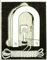
This unit has a full floating armature, which means that armature is mounted so that it acts like a plunger between two sets of magnets or pole pieces. As the magnetization of the armature changes under the influence of the signal it plunges first toward one pair of pole pieces and then toward the
