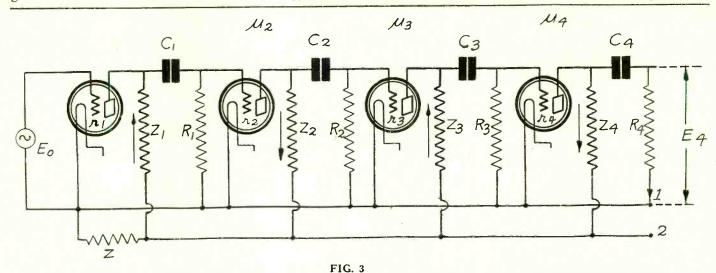
A FOUR TUBE RESISTANCE COUPLED AMPLIFIER ILLU STRATING HOW THE SIGNAL CURRENT IN THE PLATE OF THE LAST TUBE WHEN FLOWING THROUGH Z CAUSES A DEPRESSION IN THE AMPLIFICATION AND INCREASING THE STABILITY. TWO METHODS OF CONNECTING THE SPEAKER ALSO SHOWN.
