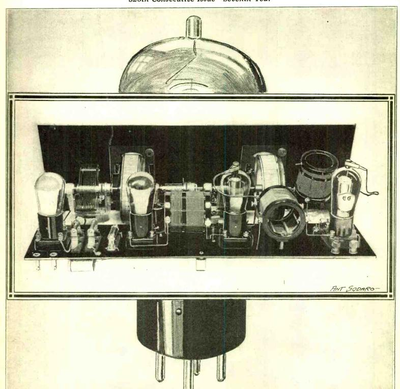
The heart of the High Mu Tuner is the screen grid tube. Two such tubes are used as radio frequency amplifiers. The detector is a high mu tube, used as a grid bias detector. See the constructional article beginning on page 3.
