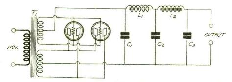
THE CIRCUIT DIAGRAM OF A B BATTERY ELIMINATOR IN WHICH TWO TYPE —80 RECTIFIER TUBES ARE CONNECTED IN PARALLEL TO IMPROVE THE VOLTAGE REGULATION OF THE CIRCUIT. CIRCUIT REQUESTED BY ROGER W. NORTON
