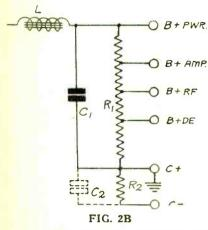
A SECTION OF THE CIRCUIT DIA-GRAM OF A B BATTERY ELIMI-NATOR SHOWING THE PROPER CONNECTION FOR LEAST HUM. THE FINAL CONDENSER CI, C CONNECTION FOR LEAST FORM.
