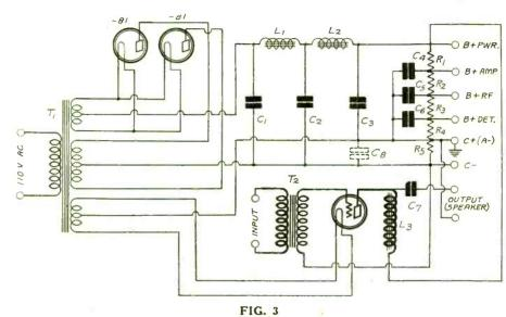
WHEN A FULL WAVE TWO TUBE RECTIFIER IS USED THE LAST FILTER CONDENSER, THE LOUD SPEAKER RETURN AND THE GROUND SHOULD BE CONNECTED AS SHOWN IN THE DIAGRAM FOR LEAST HUM, BEST LOW NOTE REPRODUCTION AND LEAST TENDENCY TOWARD MOTORBOATING.
