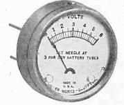
This 0.6 voltmeter, No. 306, is especially useful for the No. 25 and No. 28 Radiolas, because it is equipped with pin jacks which fit into the plugs with which those sets are provided. The meters may be used in any home-constructed set, too, where the builder desires to place tip jacks on the front panel, so the meter can be plugged in for obtain-ing reading. The meter may be kept permanently in circ ouit, if desired. No. 306, 0-6 volts DC.....
