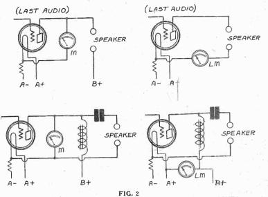
FIG. 2 HOW A HIGH RESISTANCE METER M SHOULD BE CONNECTED AS A DISTORTION TESTER. NOTE THE DIFFERENT METHOD FOR USING A RELATIVELY LOW RESISTANCE METER FOR THE SAME PURPOSE. FILTERED AND UNFILTERED OUTPUTS ARE SHOWN.
