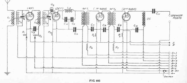
A FOUR TUBE SET SIMPLE TO TUNE AND WHICH HAS GOOD SENSITIVITY, DUE LARGELY TO SELF-REGEN-ERATION CONTROL OF THE FIRST TUBE
