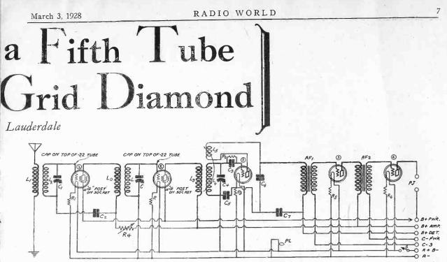
THOSE WHO HAVE BUILT THE FOUR TUBE SH IELDED GRID DIAMOND OF THE AIR AND WHO DE-SIRE TO ADD A FIFTH TUBE, SO AS TO INCREASE THE RECEPTION RANGE ABOUT 500 MILES, MAY DO SO BY MAKING THE FIFTH TUBE THE SECOND RADIO FREQUENCY AMPLIFIER. THIS IS SHOWN ABOVE AS A SCREEN GRID TUBE. (5) THE CHANGE IS EASILY MADE.
