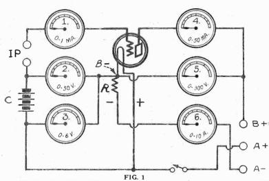
FIG. 1 FIG. 1 A DIAGRAM SHOWING THE CONNECTIONS OF METERS IN A COMPLETE TUBE AND CIRCUIT TESTER. NOTE THAT  $B_{--}$  IS CONNECTED TO FILA-MENT MINUS. THIS AVOIDS A VOLTAGE DROP DUE TO B CURRENT THAT OTHERWISE WOULD FLOW THROUGH THE FILAMENT RESISTOR R. SOME TUBE TESTERS CONNECT TO A PLUS, INSTEAD OF F-, AND THIS IS SATISFACTORY, TOO.
