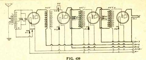
The circuit diagram of the 4-tube receiver requested by Henry Georges
