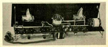
THE REAR VIEW of the New and Improved Diamond of the Air. The antenna coupler is at right (Bruno No. 99RF). Note socket strip support is on the AFT.
