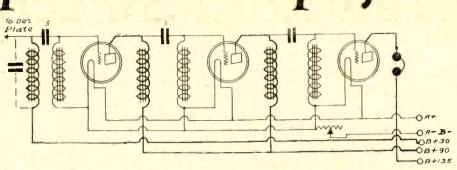
FIG. 1 The double impedance audio amplifier. The coupling condensers are 0.5 mfd. each. The grid returns, shown at negative F, may be placed instead at negative A (the other side of the rheostat) if greater "free bias" is desired.
