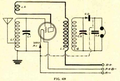
The circuit diagram of the 1-tube reflex desired by Wallace Kingle.
