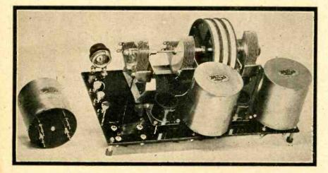
VIEW of the Welty RF unit, showing the interchangeable RF coils and the localized control tuning. Note the rugged construction of the sub-base. A coil with the four terminals at the base is shown to the left.
