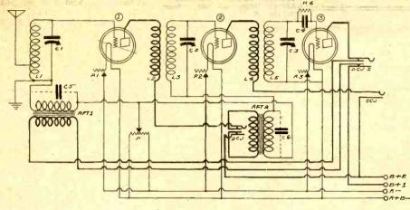
A 3-TUBE reflexed receiver, wherein the two RF tubes act both as RF and AF amplifiers, in conjunction with a non-regenerative detector.
