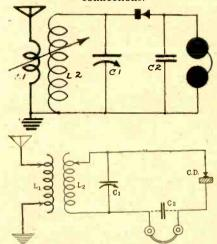
CIRCUIT DIAGRAMS of two selective and voluminous crystal receivers. Inductive coupling is used in the top diagram while conductive coupling is used in bottom one. An antenna coil having a variable primary may be used in the upper circuit, while an RFT with a large primary (20 turns) tapped at every second turn, should he used below.
