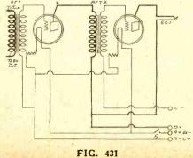
The circuit diagram of the 2-step AF amplifier.
