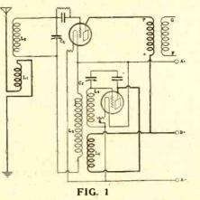
L2 is hooked up to the modulator tube and L4 to the Oscillator tube. C1L2 is tuned to the station's frequency and C2L4 to a frequency differing from the station frequency by the intermediate frequency. L3 is common to both circuits.
