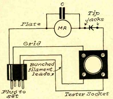
AN OLD socket base, connected up as above, may be used as an efficient tube tester. MA is the milliammeter Tip jacks afford a listening post.
