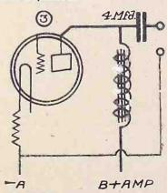
HOW TO hookup an impedance and a fixed condenser to the output of the last AF power tube to keep DC off the speaker.
