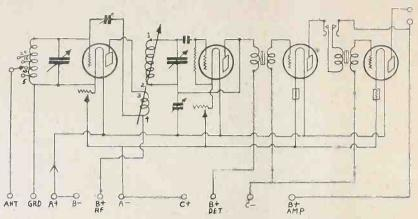
FIG. 421 Circuit diagram of a 4-tube set that has a tuned impedance input circuit , with a tapped aerial coil.
