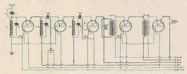
A 5-tube receiver, employing two stages of impedance coupled radio frequency amplification, a non-regenerative detector and two stages of transformer coupled audio frequency amplification. A potentiometer is used in the grid return of the second RF tube for controlling the oscillatory action of this tube. Then ohm rheostats are used in the RF and AF filament circuits. A 20 ohm rheostat is used in the detector filament circuit.
