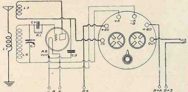
HOW A 2-stage A-K transformer coupled audio frequency amplifier may be hooked to the output of a regenerative tube detector is shown above diagrammatically. The filaments of the AF tubes are singularly controlled. The standard transformer hookup is used in the unit. Higher B voltages than those marked on the unit may be applied.
