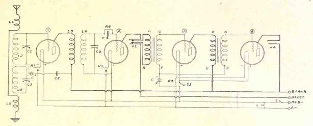
FIG. 1. An unusual method of employing the acceptor method of tuning (C3. L4), although at first blush it looks like a rejector wavetrap, is shown above. The amplification is at least doubled and selectivity enhanced greatly. The winding L5 is an important factor in the system.
