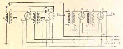
THE TICKLER COIL is used in both the radio frequency and detector stages by the method shown in the diagram. The method is a departure from the conventional in hookups, and is suggested by the author as a means of remedying critical tickler adjustment.
