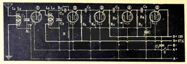
THE ELECTRICAL diagram of the 2-C, 5-tube receiver, described in the January 2 issue of RADIO WORLD by Capt. P. V. O'Rourke. L1 and L3, the primaries shown by the heavy white lines, are wound in the middle of the secondary and side by side with the continuation of the secondary winding. The secondary, using .00035 mfd. variable condensers, consists of 65 turns on 3" diameter.
