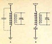
IN A we have one method of increasing the wavelength of an antenna, by the insertion of a fixed condenser in shunt to the antenna and the ground. This has the same effect in some instances as adding turns to the secondary or increasing the physical length of the antenna. In B we have a method of decreasing the wavelength of the aerial by inserting a fixed condenser in series with the ground lead. In both instances the condenser should be of small capacity, say not more than .00025 mfd.
