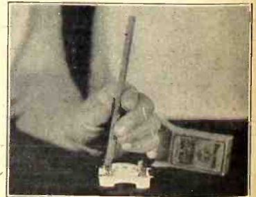
WORKING IN receivers, where sockets, etc., are very close to each other, makes it difficult to place thumb nuts on the binding posts. This can be remedied by forcing a lead pencil tip into the nut. It is thus started. A pair long nose pliers can tighten the nut up. (Hayden)
