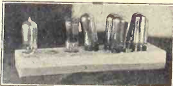
A SMALL candy cardboard box may be employed as a tube rack. Tubes which have been removed from the set may then be placed in holes, punched or cut to the specific size of the bases of the tubes, instead of placing on the table and taking a chance of them being knocked off.
