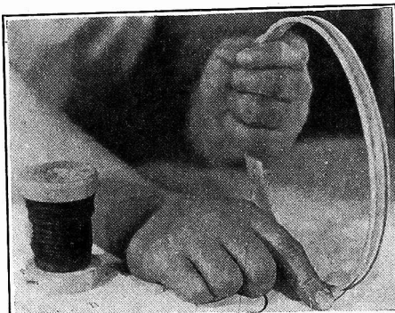
FIG. 3—Now begin the winding, using the method shown. Put in 12 turns of No. 22 double silk covered wire.
