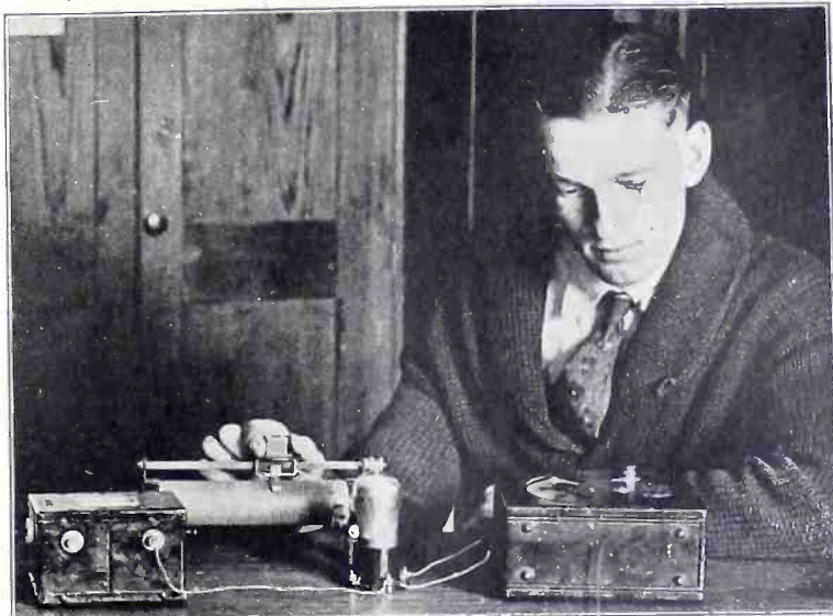
R. P. BATTLE, of the Radio Laboratory of the Bureau of Standards, reactivating an XL (Thoriated) filament electron tube. The transformer changes the 110-volt alternating current to the proper voltage for reactivation as indicated by the voltmeter. This process consists of boiling additional atoms out of the interior of the tungsten filament. This forms a new layer of thorium atoms on the surface. The boiling is done by operating the filament for a very brief interval at a specified high voltage followed by a low voltage. (Harris and Ewing.)
