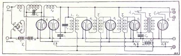
A FIXED bypass condenser across the B battery is shown above (C), to right of C4, a bypass condenser for RF currents (to right of second tube from left) should not exceed .002 mfd. The intermediate frequency condensers in the above Super-Heterodyne are C3, to right of second tube, across primary, and the ones across succeeding secondaries. (Fig. 4.)
