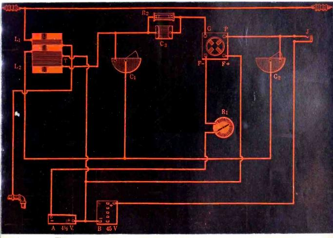
THE 1-TUBE SET wiring is shown above in picture form. See article on page 16.
