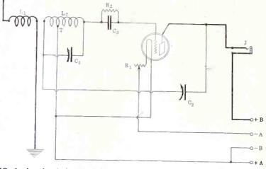
FIG. 1, the electrical wiring diagram of the Bernard 1-tube DX set, shown schematically. The coils are drawn in such fashion as to clarify the manner of connecting their terminals and the tap T. Regeneration is supplied by the Hartley oscillator hookup, the same system as used by Bernard in the Thordarson-Wade 5-tube set. Note that the rotors of both C1 and C2 are connected to the same lead that goes to the beginning of the secondary L2, and this lead connects nowhere else.
