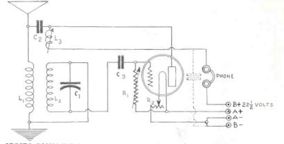
SERIES COUPLING by means of a fixed condenser, C2. (It should be very small, say .0001 mfd., for loose coupling and large (e.g., .002 mfd.) for tight coupling. Fixed condensers used, as C2, in RF work, should have only the best dielectric. C3 is the grid condenser, used for blocking the grid current in the detector. The dotted condenser is a bypass. (Fig. 1.)
