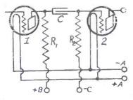
A FIXED condenser, C, used somewhat similarly to a grid blocking condenser. The above is a direct coupled circuit, tubes 1 and 2 being coupled by condenser, with the aid of resistors, for audio amplification. For such audio coupling C should be as large as bossible. The large condensers are expensive, so .25 mfd. is a frequent compromise, yet 4.0 mfd. would be much better. The reasons are given in the text. (Fig. 2)
