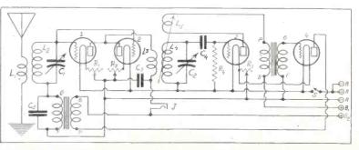
C3. BETWEEN the end of L3 and the A minus lead, to lower right of the second tube, is used as a bypass. C5 is also a bypass condenser in its conventional position on a reflex set, across the secondary of the first AFT (lower left). Bypass con-densers should be no larger than necessary. (Fig. 3.)
