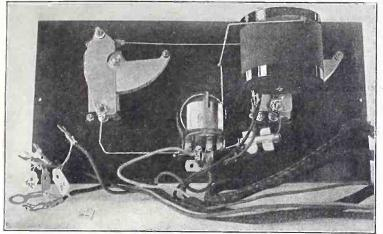
THE REAR VIEW of the set, showing the tap lead that goes to A+.
